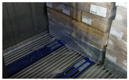
Image 4: Roller forks being slid under the slip sheet pallet
