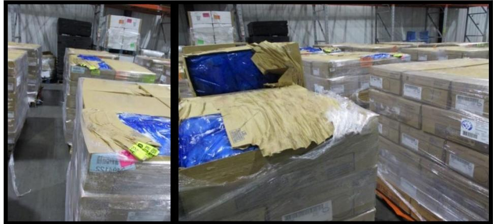
The images shown in Figure 16 are from the pallet pilot and show the damage that can be done without having a slip sheet on the top of the crate. Pallets must have slip sheets placed on the top and bottom of the pallet (see Section 4.2.2).
